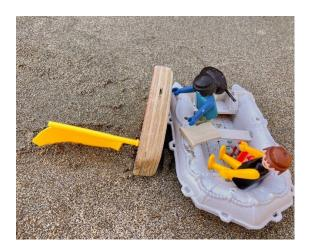
When the opti is nearly over, you will need to remove the centreboard and grab the gunwhale to push opti down to rest of the way, don't let go until the opti is upright.)
