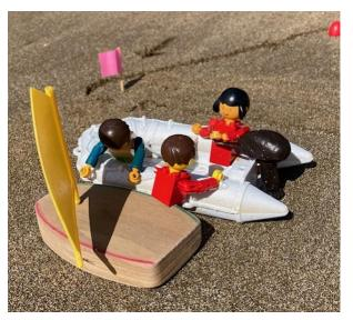
Patrol Boat waits for the Opti to slow, with sail flapping, and comes alongside the Opti on the **WINDWARD** side. The boat handler keeps the boat going slow, with just enough speed to keep the Opti in this position (with the sail well out of the way).
